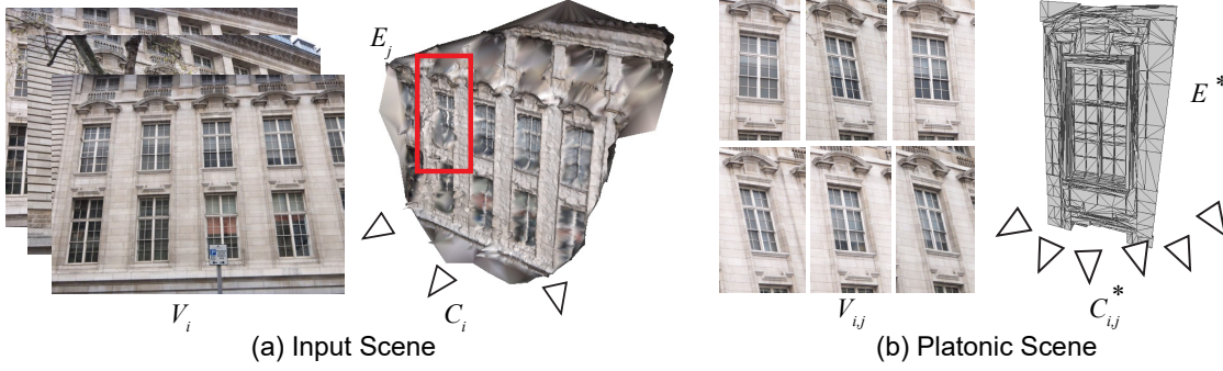
Figure 3.4 – From given input views V_i of a facade and their associated cameras C_i (a), we extract subviews V_{i,j} of similar windows E_j . From these, we can reconstruct a 3D model of the platonic element E^* along with platonic cameras C_{i,j}^* (b) in a common space.
