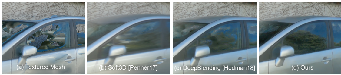
Figure 4.1 – We propose a new solution for rendering captured cars, and in particular their reflective, semi-transparent windows. A textured mesh from multi-view stereo reconstruction (a) is missing the window geometry. Recent free-viewpoint Image-Based Rendering algorithms (b, c) are not designed to handle the rendering of both the reflection of blue sky, green leaves and the transmissive content (car interior). Our method (d) handles this by computing real-time reflection flows on an ellipsoid approximation of the curved window surface, based on our estimate of a smooth hull of the car that exploit semantic labels in the input images.
