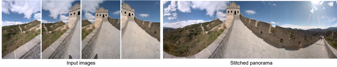
Figure 2.4 – Multiple images taken at the same location can be combined to generate a panorama. The user can freely rotate around to visualize the scene.
