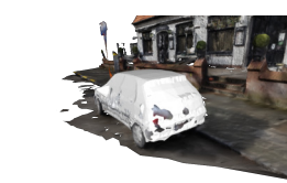
Figure 1. Overview. We propose a new method for Image based rendering that takes advantage of 3D model databases. At a fully automatic Preprocessing stage, (1.a) cameras are calibrated and 3D reconstruction is estimated using multi-view stereo [25]. Objects of interest (here cars) are detected using R-CNN[16]. These detections are matched using viewing rays in cyan. (1.b) The corresponding images are used to query our database of 3D objects, (1.c) which returns a 3D model and an orientation relative to the cameras. (1.d) Combining depth and silhouette cues in multi-view, (1.e) a better alignment of the object is obtained. During Rendering , we generate the novel viewpoints illustrated by the blue camera (1.a). State of the art methods (e.g., [38]) exhibit strong artifacts on the car (2.a). Using our approach (2.b) we achieve good rendering quality for both the car and the background.
