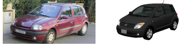
Figure 4. Model and orientation matching. The detection algorithm provides 2D bounding boxes for the object. After cropping, the images are used to query the database. Right: the matched rendering which provides both a 3D model and an orientation.
