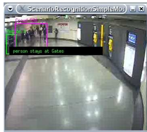
Figure 2: A person and a crowd are tracked. The event ‘person’ stays at gates has been detected.
