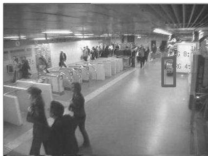
Figure 6. The new scene object is detected as a stationary region represented by a blue bounding box.
