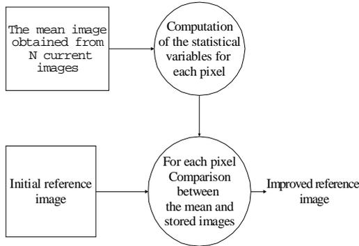
Figure 2. Overview of the algorithm to improve the reference image
