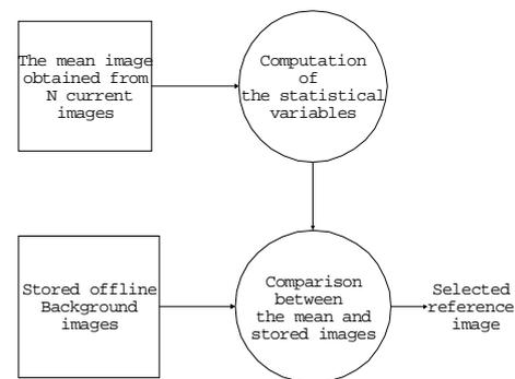
Figure 1. Overview of the algorithm to initialise the reference image
