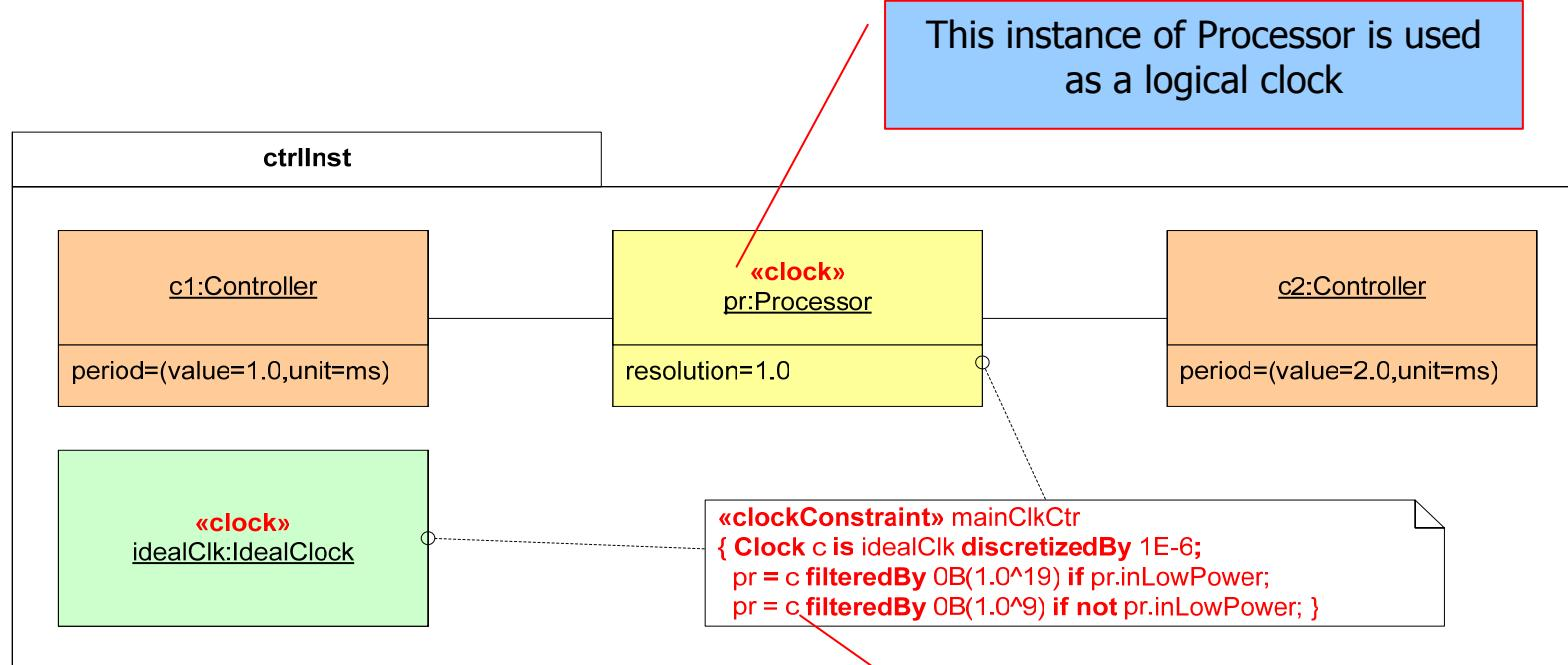
This clock constraint binds processor clock cycle to physical time, taking account of the power mode
