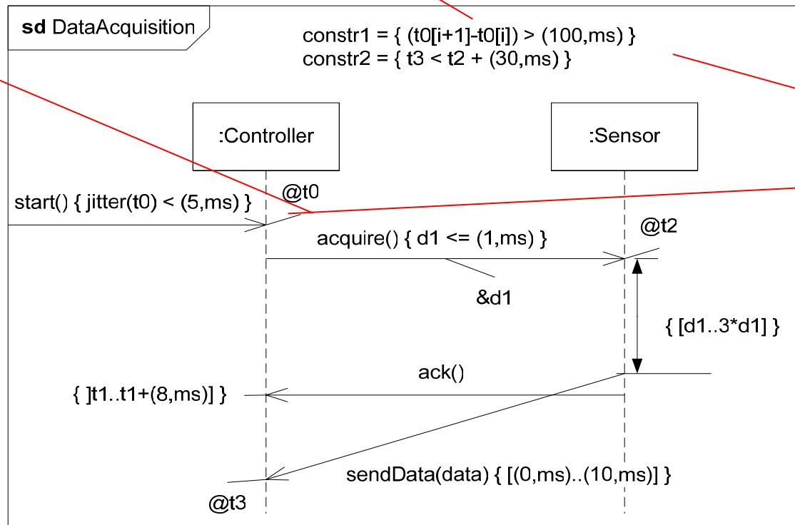
$t_0$  is periodic, period 100ms with a jitter less than 5ms
