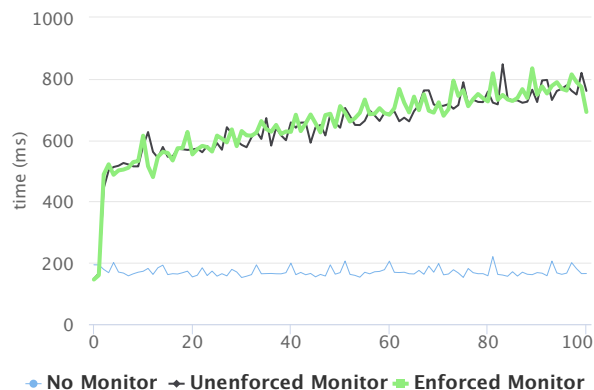
Figure 2: Performance overhead of deploying the monitor. As one can observe, there is an observable overhead due to the use of service workers themselves ( No Monitor vs. Unenforced Monitor ). However the implementation of our monitor within the service worker itself induces very little overhead ( Unenforced Monitor vs. Enforced Monitor ).
