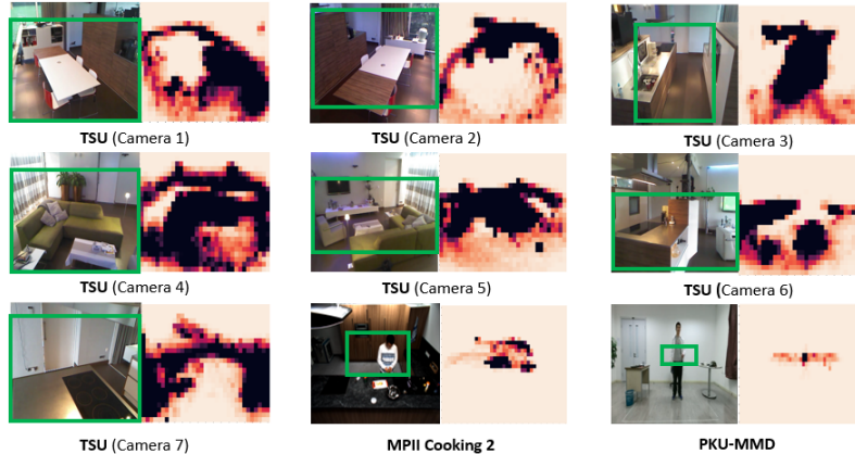
Figure 3-6: Spatial Distribution of the person location in normalized image coordinates for 3 datasets, dark regions correspond to high frequency areas of the person position. The green bounding boxes embrace the high frequency locations. From the size of the bounding box, we find that TSU exhibits the largest spatial scatter, indicating the low camera framing property.
