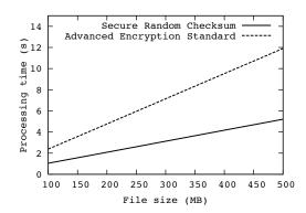
Fig. 3. File processing time versus file size with SRC and AES
