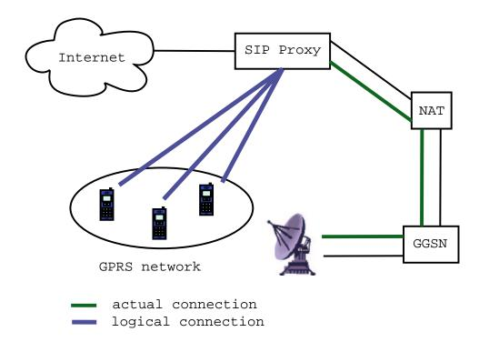
Figure 5.2: SIP proxy for connectivity through NAT for GPRS network
