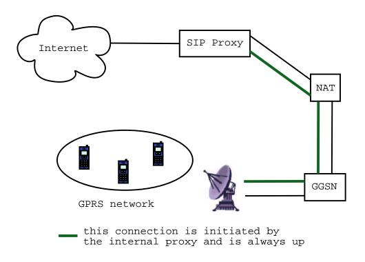
Figure 5.3: GPRS network enabled for constant SIP connectivity using SIP proxies
