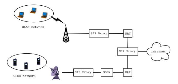
Figure 5.4: GPRS and WLAN networks for SIP communication
