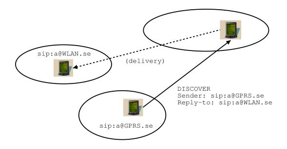
Figure 6.8: Redirection of content delivery to different interface
