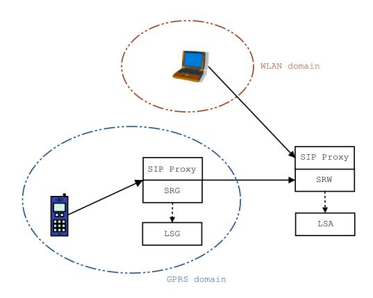
Figure 5.7: Hierarchical structure of SIP Servers for heterogeneous networks
