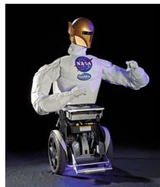
**Figure I.7** – The NASA Robonaut consists of an upper body placed on a wheeled mobile base
