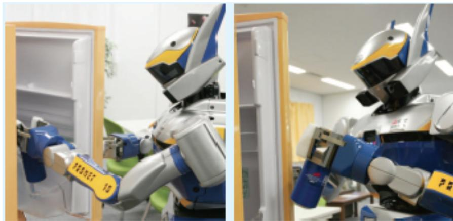
**Figure I.10** – A work at AIST with the HRP-2 humanoid has combined high-level teleoperation with autonomous perception and control. [SSY<sup>+</sup>06]
