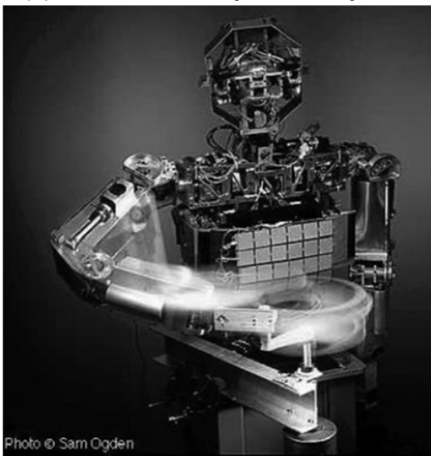
(c) Upper limb robot with SEAs [Brooks 1999].
