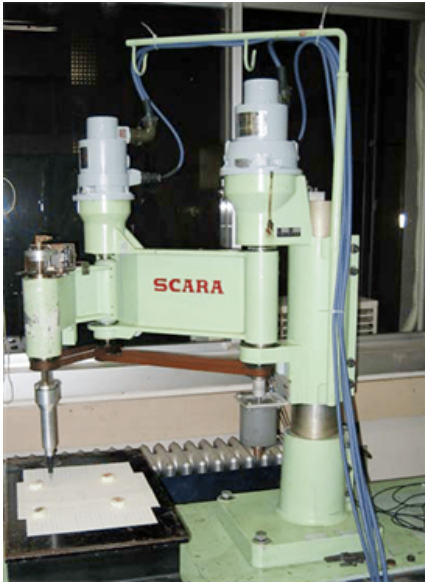
(a) First prototype of SCARA robot [Makino 1980].
