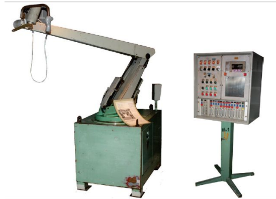
(b) First commercial painting robot in 1969 [IFR].
