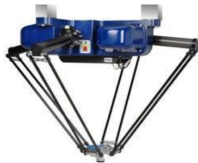
(b) H4 robot with asymmetrical design [Pierrot 2001].
