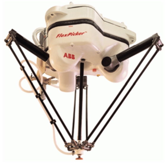
(b) The Flex-Picker robot from ABB [Pierrot 1999].
