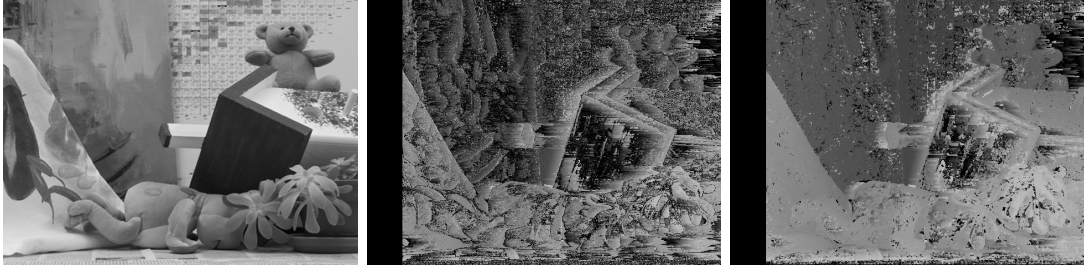
Figure 4.3: An example of a naive approach to stereo correspondence. From left to right: reference image, disparity based on a single pixel brightness, disparity computed using 3 \times 3 pixel descriptors. The stereo image is taken from Scharstein and Szeliski (2003).
