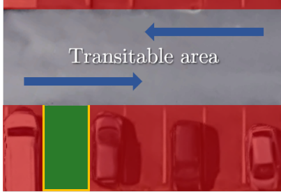
Fig. 3. Example of a parking environment. The green rectangle denotes the parking spot into which the car should park. Red areas are considered forbidden zones, as such the vehicle should never go into them. Furthermore, it is considered that parking maneuvers can only start inside the transitable area and if no portion of the vehicle is inside any of the forbidden zones.
