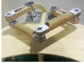
Figure 3: Final prototype of a wooden five-bar mechanism.
