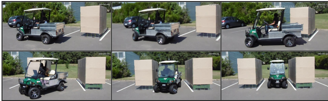
Fig. 13: Evolution of the sensor based perpendicular parking maneuver
