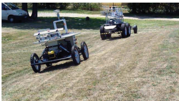
Figure 11. The off-road robots in formation with RobuFAST leading Arocco.
