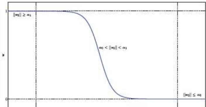
$$w = \begin{cases} 1 & \text{if } ||e_2|| \geq \alpha_1 \\ \frac{1}{1 + \exp\left(20 \frac{||e_2|| - \alpha_1}{\alpha_0 - \alpha_1} - 10\right)} & \text{if } \alpha_0 < ||e_2|| < \alpha_1 \\ 0 & \text{if } ||e_2|| \leq \alpha_0 \end{cases}$$
