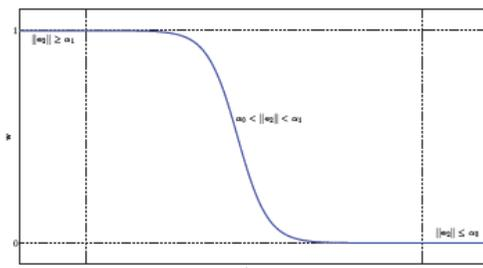
$$w = \begin{cases} \frac{1}{1 + \exp\left(20 \frac{\|e_2\| - \alpha_1}{\alpha_0 - \alpha_1} - 10\right)} & \text{if } \|e_2\| \geq \alpha_1 \\ \frac{1}{1 + \exp\left(20 \frac{\|e_2\| - \alpha_1}{\alpha_0 - \alpha_1} - 10\right)} & \text{if } \alpha_0 < \|e_2\| < \alpha_1 \\ 0 & \text{if } \|e_2\| \leq \alpha_0 \end{cases}$$
