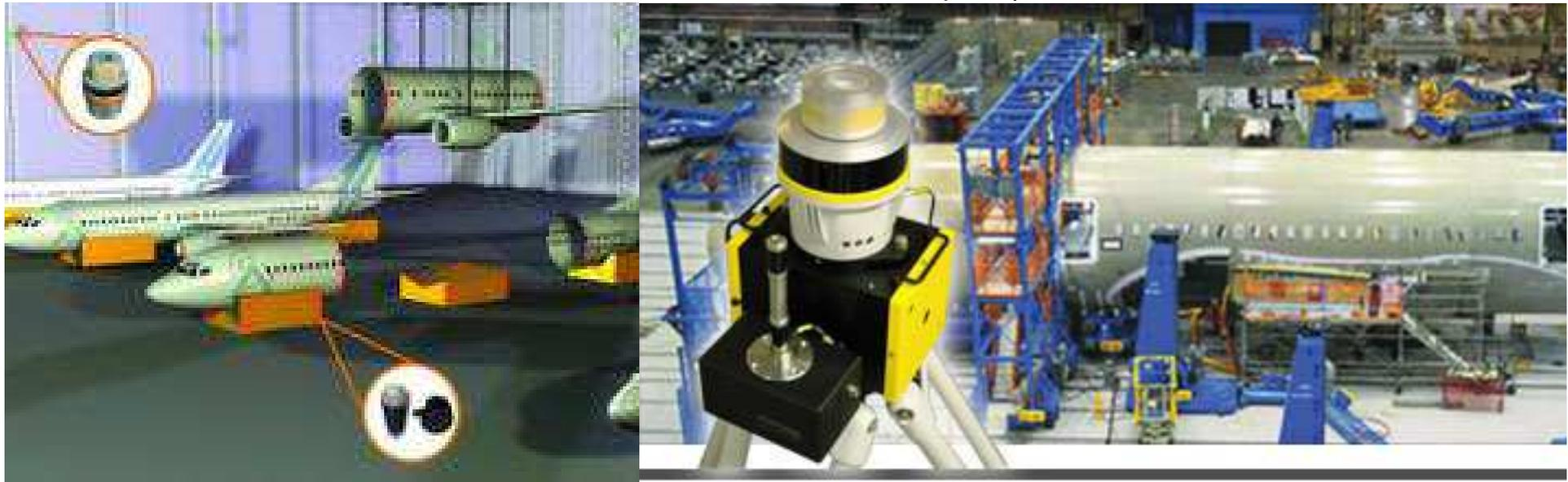
**iGPS system is comparable to a GPS. GPS satellites are replaced by infrared iGPS laser transmitters that activate a measurement field as large as an entire room or facility.**
