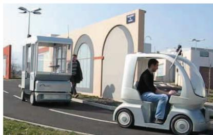
Fig. 1. Experimental vehicles: a Cycab leading a RobuCab
