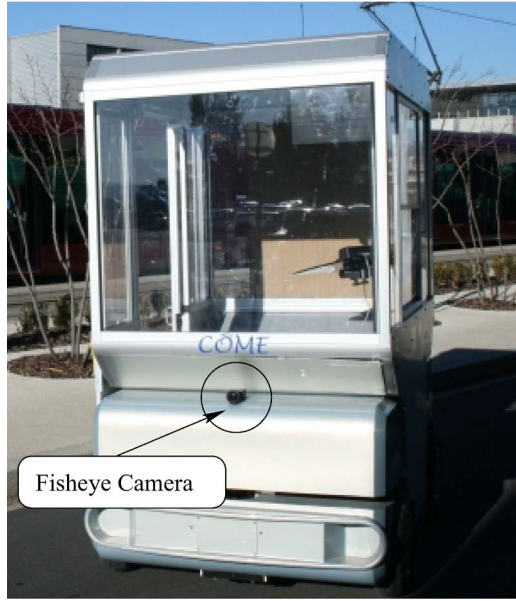
Fig. 7. RobuCab vehicle with the embedded camera.
