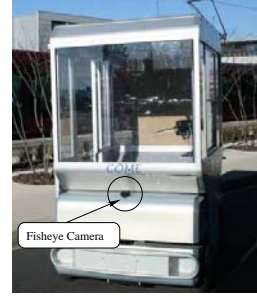
Fig. 7: RobuCab vehicle with the embedded camera.
