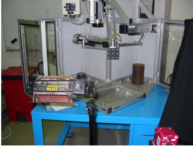
Fig. 1. Experimental set-up: the Orthoglide is observed by a high-speed camera.
