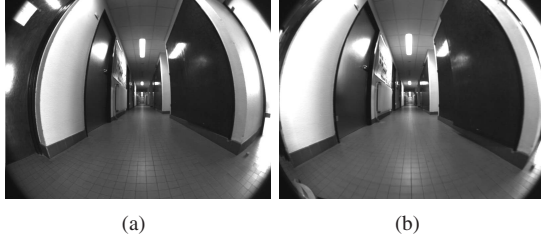
Fig. 5. Result of the localization step: the current image (a) and the nearest key image (b) have 306 matched points.
