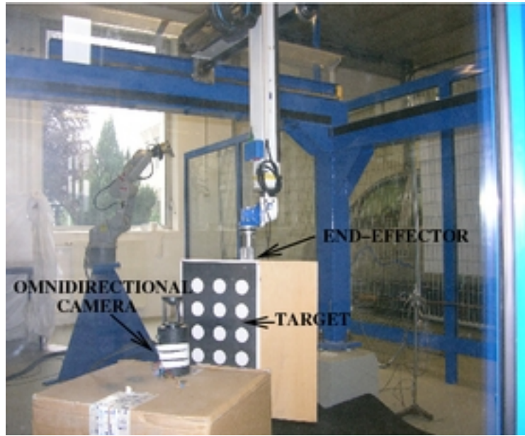
Fig. 6: Experimental setup : eye-to-hand configuration
