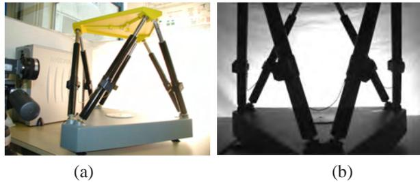
Fig. 1. A Gough-Stewart platform observed by a classical perspective camera: (a) camera position with respect to the platform legs, (b) leg images
