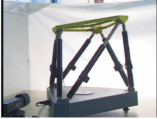
Fig. 3. Experimental set-up: A Gough–Stewart platform observed by a camera.
