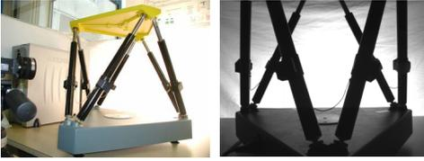
Fig. 2. A Gough-Stewart platform observed by a perspective camera.
