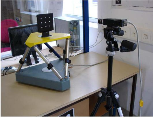
Fig. 8. A Gough-Stewart platform observed by a camera.
