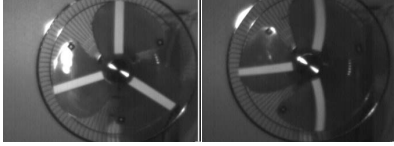
Fig. 2. An example of distortion of a rotating ventilator observed with a Rolling Shutter camera: static object (right image) and moving object (left image).
