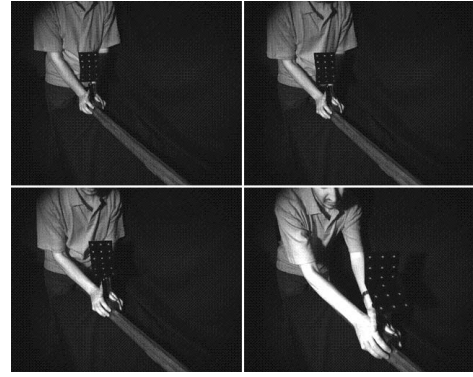
Fig. 4. Image samples of pure translational motion.
