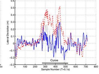
Fig. 10. Lateral deviation of path #2 with real measurements
