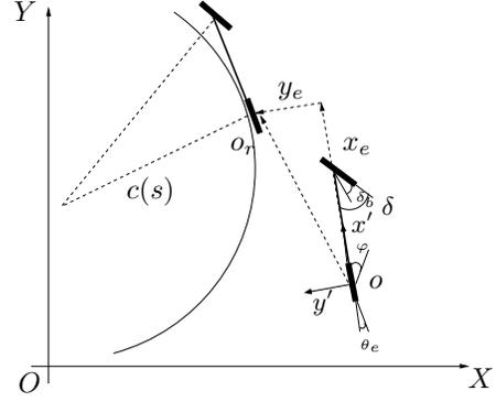
Fig. 1. Notations of the kinematic model
