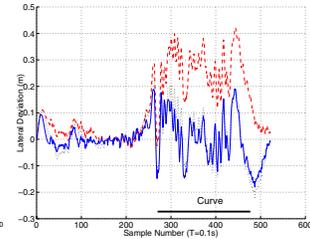
Fig. 7. Lateral deviation of path #1 with real measurements
