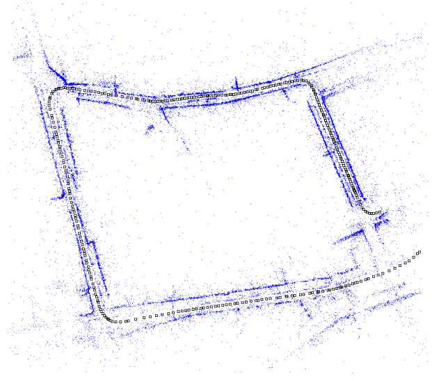
Fig. 9. An example of Vision based memory of a reference trajectory
