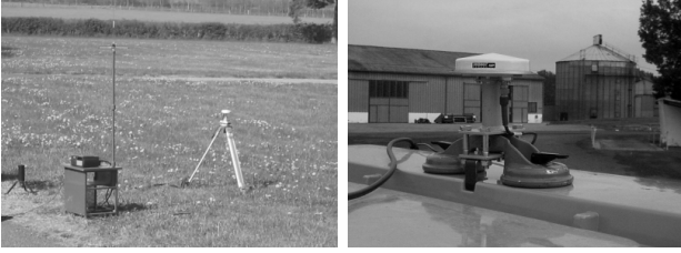
Fig. 2. RTK GPS main sensor implemented on vehicle
