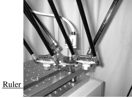
Figure 13: Validation experiment - Kinematic constraint on the end-effector
