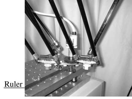
Fig. 5 : Validation experiment - Kinematic constraint on the end-effector
