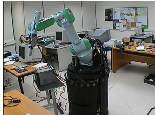
**Figure 3:** The stereo visual servoing manipulator setup.
