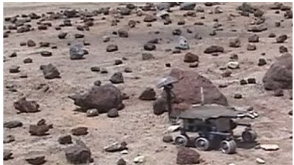
Fig. 1. FIDO rover navigates autonomously using the proposed motion planner among dense obstacles in the Mars Yard at the California Institute of Technology, Jet Propulsion Laboratory. The planner manages frequent updates of the limited perception system by replanning continuously at approximately 10Hz. Computed planner motions are smooth in curvature and executable by the robot verbatim.
