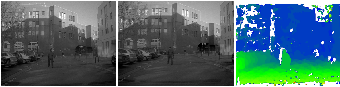
Fig. 1. Left image, right image and corresponding disparity map
