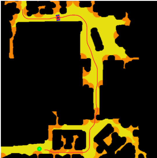
Fig. 5. The 'long run' encompasses a path of approximately 40[m] through the Intel Research Pittsburgh lab. The 3D planner expands less than 100 states in 0.04[s] to arrive at a solution. The 4D planner takes 2.28[s] with 5900 expanded states (pictured). The large difference in performance lies in the 2D heuristic, which does not well predict the influence, which areas of reduced maximal velocity (i.e. in vicinity of doors and narrow hallways, colored orange) have on the 4D planner.
