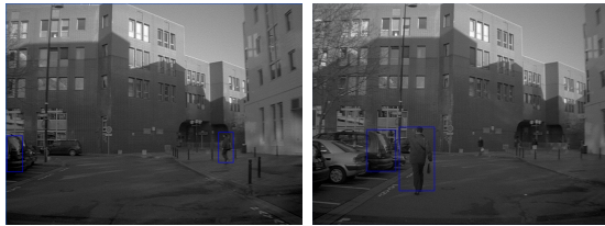
Fig. 5. Some false alarms on the back of partly occluded parked cars.
