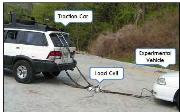
Fig. 9. Experiment to measure friction coefficient
