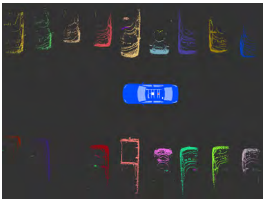
Fig. 7. Segmentation of obstacle points within the scene. Different colors represent different segmentation groups. Good obstacle discrimination simplifies obstacle segmentation.
