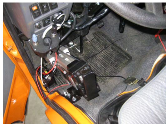
Fig. 9. The linear actuator installed on-board of the vehicle.
