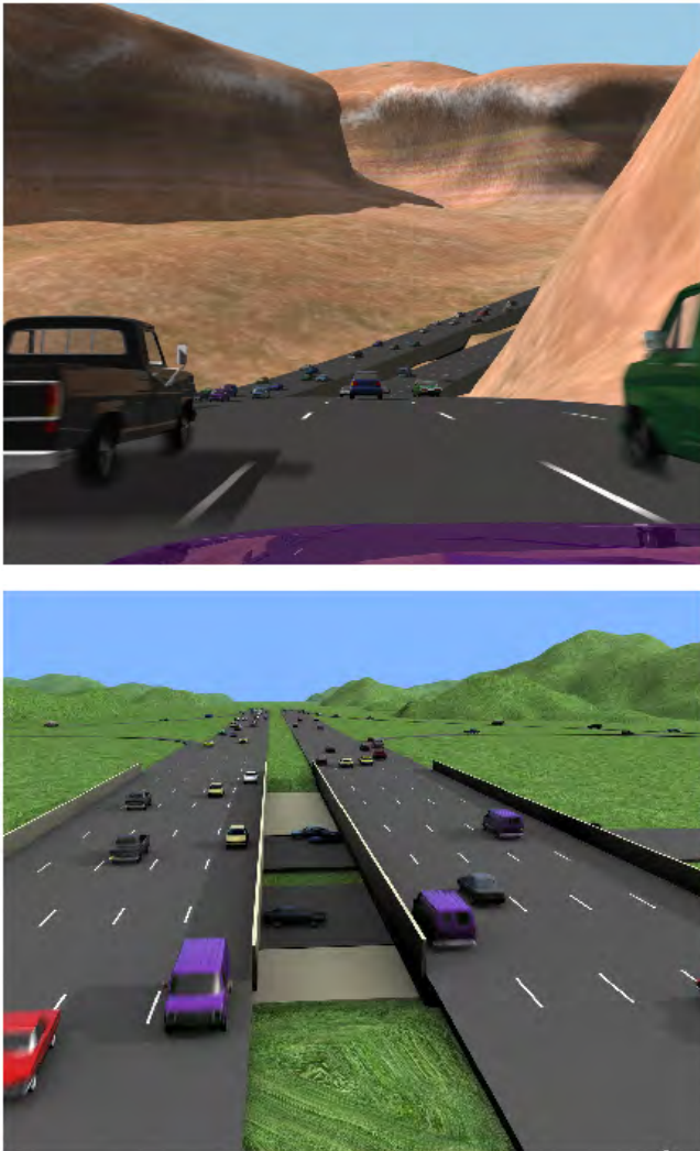
Fig. 1. Images of highway traffic synthesized by our method. Our method computes trajectories one by one for a continuous stream of cars (of possibly high-density). The trajectories fit the boundary conditions at the sensor points, and obey the geometric, kinematic and dynamic constraints on the cars. The number of lane changes and the total amount of (de-)acceleration are minimized and the distance to other cars is maximized to obtain smooth and plausible motions.
