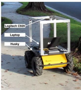
Figure 4. Clearpath Husky with a Logitech C920 for outdoor environment
