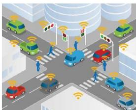
**C-ITS: Intelligent Transport Systems (ITS)** where ITS stations (vehicles, roadside equipment, traffic control centers and personal devices) communicate and share information
