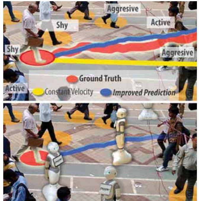
Fig. 1: Pedestrian Prediction and Multi-Robot Navigation: We developed an algorithm to predict the path of each pedestrian (i.e., close to the ground truth) and use the predicted path for collision-free multi-robot navigation. We also classify the behavior of each pedestrian from his or her trajectory and adjust some of the components of social constraints (e.g., personal space, entitativity behavior, etc.) accordingly.
