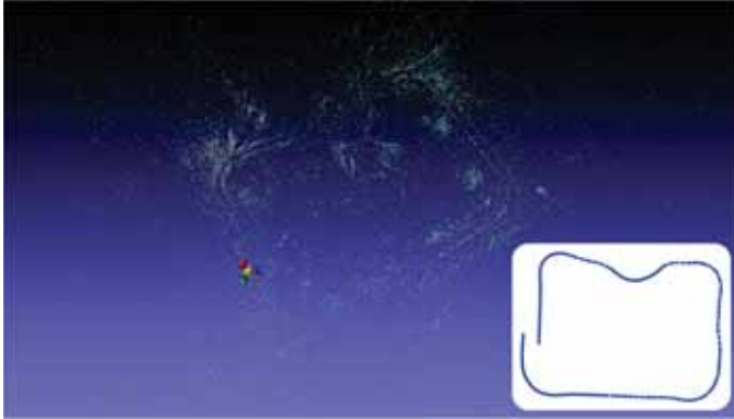
Figure 3. Reconstruction of the rigid environment generated by the visual SLAM module and its corresponding trajectory.
