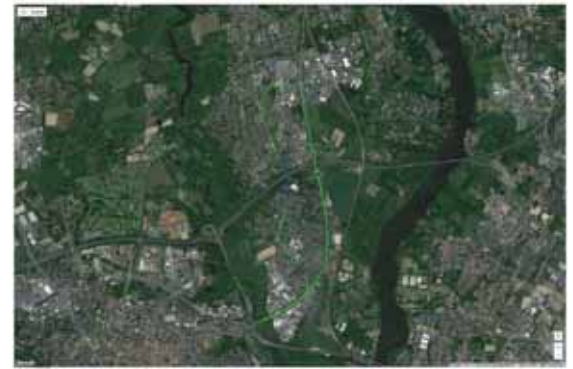
Fig. 8. RTK-GPS coverage - Residential zone (RTK zones in green)
