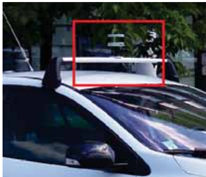
Fig. 2. The Velodyne VLP-16 on the roof of the Renault Fluence ZE.
