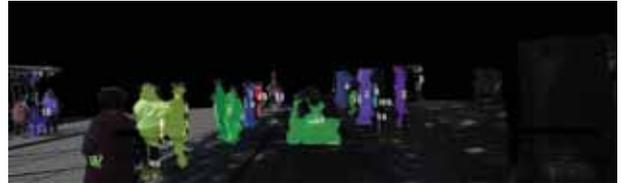
Fig. 6: Obstacles very close to the camera were not detected because of the maximum disparity parameter.
