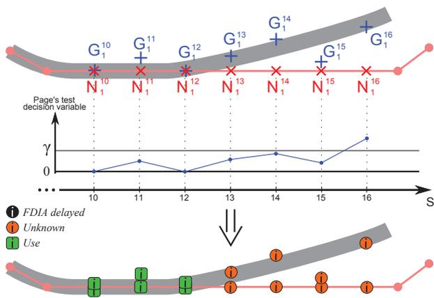
(b) Page's decision variable exceeds the threshold at  $s = 16$ . FDIA is run for abscissas 13 to 16 with  $r_{G_1 N_1} = 1$ . This results in *Knowledge of fault: Unknown*.
