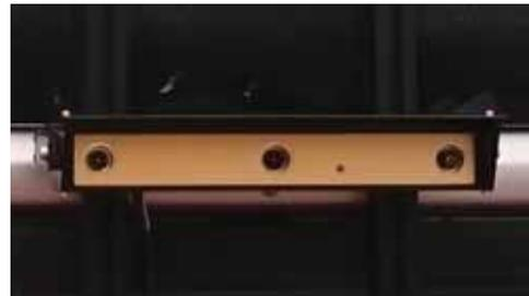
Fig. 7: The images were captured by the extended baseline of a Bumblebee XB3 Point Grey.
