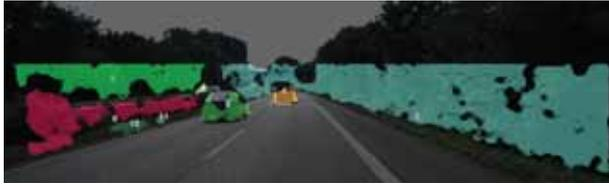
(a) Image from KITTI object detection benchmark. Four of the five visible cars were detected (2, 3, 4 and 5). One car was wrongly clustered together with the guardrail.
