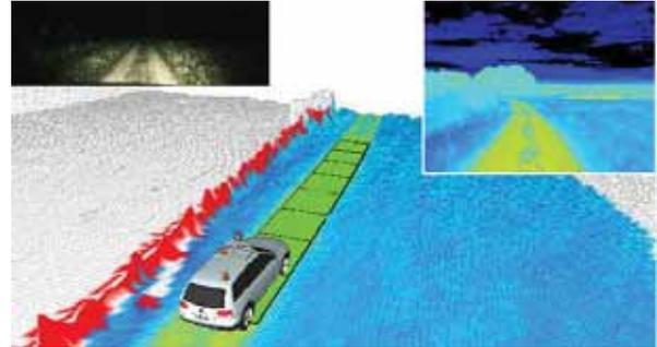
Fig. 1. Tracking a rural road at night using a multi layer terrain map (thermal layer is shown). Red cells indicate obstacle cells. Upper left: Color Night Vision camera, Upper right: thermal camera
