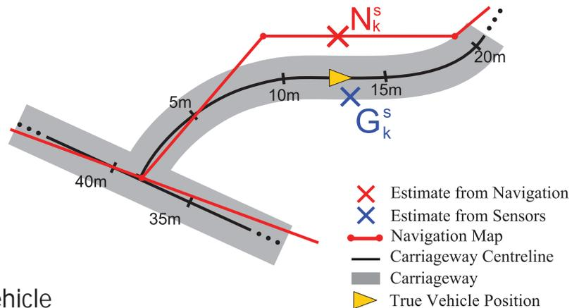
FDIA is based on the comparison of vehicle position estimates:
