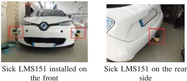
Fig. 2. The LiDARs Sick LMS151 are installed in strategical positions to ensure a 360°FoV around the vehicle.
