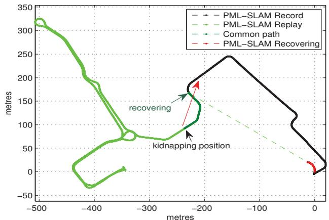
Fig. 8. Vehicle path estimated by PML-SLAM during experiment in mapping with kidnapping and recovering from kidnapping.
