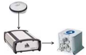
GPS + IMU as ground truth
