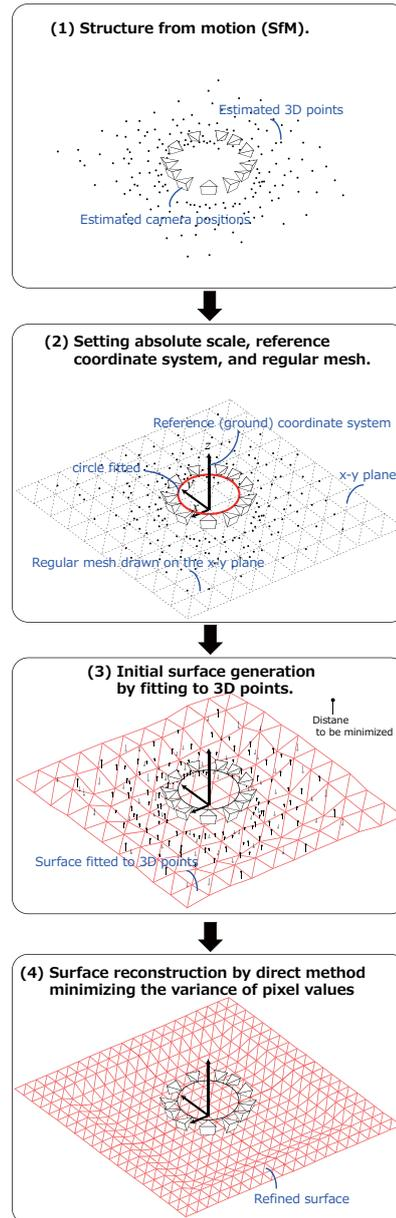
Fig. 2. Algorithm flow.
