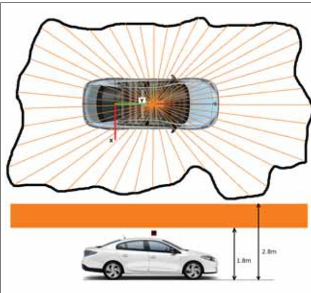
Fig. 5. Sensor configuration for Fluence. A  $360^\circ$  laser scan is obtained from the 3D point-cloud generated with VLP-16. In the bottom, the profile point-cloud range involved in the generation of the planar scan is shown.
