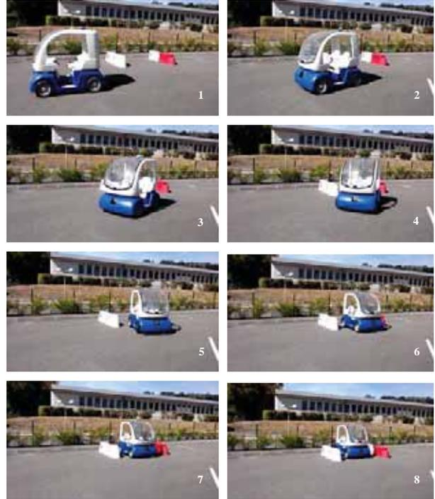
Figure 8. Automatic perpendicular parking of a CyCab vehicle
