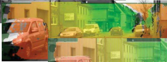
Disparity Image (SGM) 500.000 points in 3D real-time on FPGA
