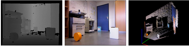
Fig. 4. Raw output of the RGB-D camera, and illustration of 3D image forged by combination of depth and color information.
