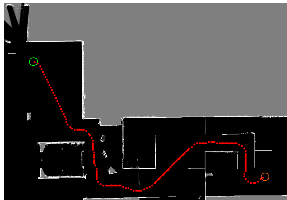
Fig. 8. Example of a planned trajectory keeping away from obstacles
