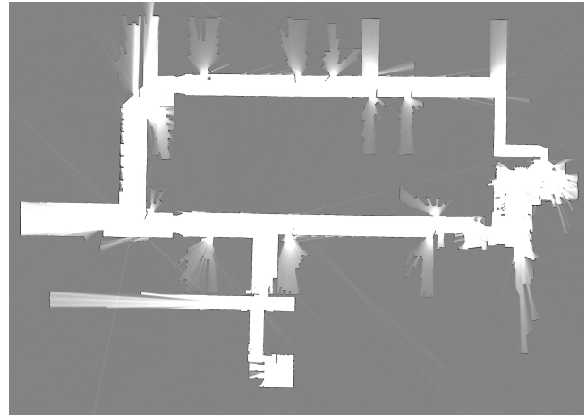
Fig. 3. Illustration of a map (63m long building) created without loop closure.
