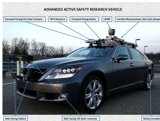
Fig. 1: TRI-NA test vehicle, showing the sensors used for various advanced safety and autonomous driving research projects. Details of the sensors used for lane mapping are in the text.
