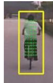
Fig.6. the Location of the Feature Points in Bicycle Tracking
