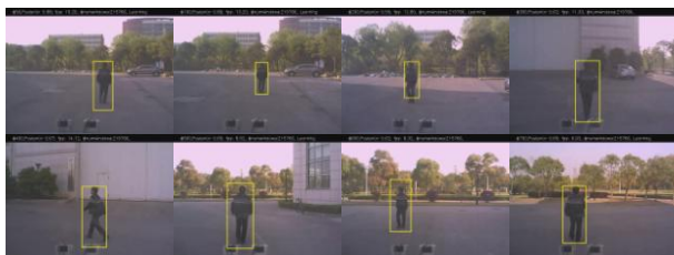
Fig. 11. The Modified TLD Algorithm Experimental Results of Test Data 2.
