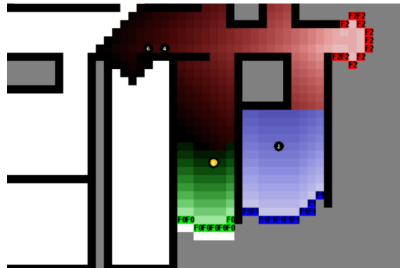
Fig. 7. Illustration . Wavefronts are stopped on the encounter of the yellow robot computing its assignment. Color code : white=explored, gray=unknown, black=walls, red-green-blue=frontier and gradient wavefront propagation result, only the wavefront closest to the frontier is shown where waves are superimposed.
