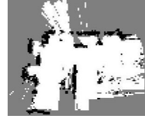
Fig. 12. Higher resolution grid - laser map - generated by best particle ( P_0 = 0.9 and E_0 = 0.5 ).
