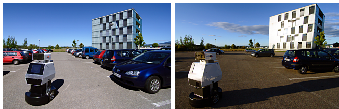
Fig. 1. A robot navigating in a parking lot at noon (left) and at 6 pm (right). Note that despite being at the same spot in both cases, the observations will be substantially different due to the changed number of parked cars.
