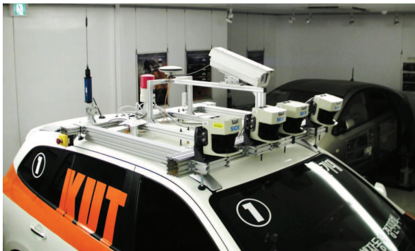
Fig. 3. View of custom made roof rack with sensors
