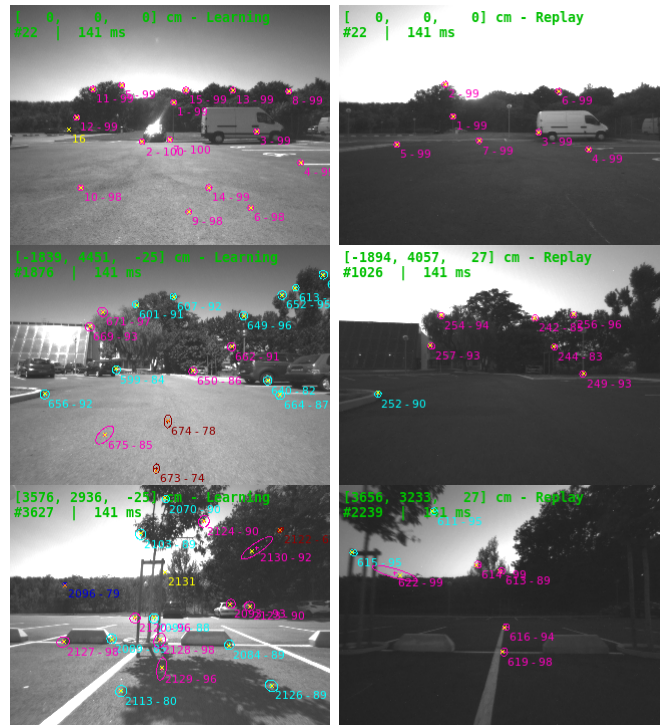
Fig. 8. Learning and Replay experiment: images acquired on the same area. (left) learning-mapping step; magenta: IDP landmarks; dark red: IDP landmarks not observed in the frame; cyan: euclidean landmarks; dark blue: euclidean landmarks not observed in the frame. (right) replay-localization step; magenta: initial projections of 3D points from the learned 3D map; cyan: projected and matched points using for localization.
