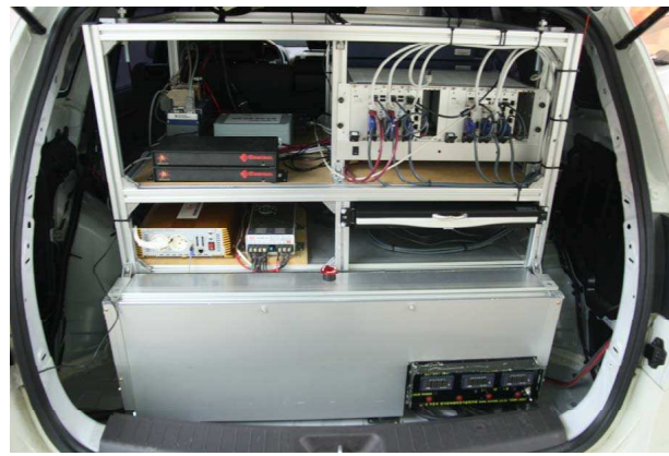
Fig. 4. Controllers and communication system in the trunk of the vehicle
