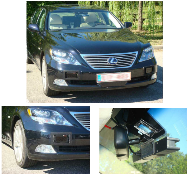
Fig. 1. Lexus LS600h car equipped with two IBEO Lux lidars and a TYZX stereo camera
