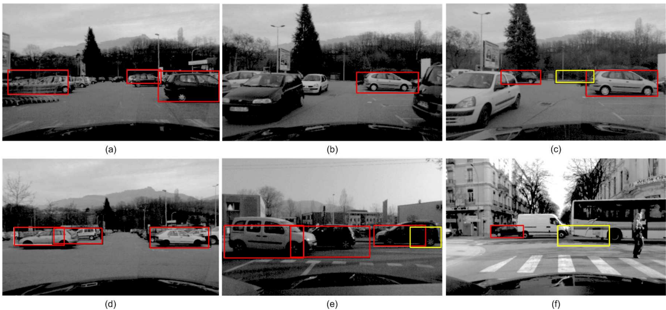
Fig. 6. Car-side detection examples. True and false positive detections are represented with red and yellow bounding boxes respectively. (a) Cars in different scales with significant background clutter and significant occlusions are detected. (b) Precise detection of the un-occluded vehicle, whereas a vehicle that is heavily occluded in the left is not detected. (c) Difficult detection of a vehicle which is far and partially occluded and a false detection in the region between the road surface and the trees. (d) Detection with partial occlusion. (e) Partial detection of a taller than normal vehicle (on the left). The training dataset does not contain vehicles of this type. (f) Successful detection of a partially occluded car and a false positive arising from a bus and a van. Training separate detectors for these types of vehicles as well will help to avoid these false alarms.
