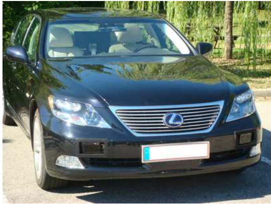
Figure 10: Experimental platform on a Lexus LS600h equipped with two IBEO Lux lidars, a TYZX stereo camera, and an Xsens MTi-G inertial sensor/GPS.
