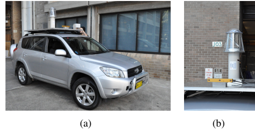
Fig. 6. (a) Test vehicle used in the experiments. (b) Radar sensor and GPS mounted on the vehicle.
