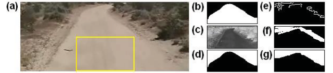
Figure 10. (a) Original image after sky removal and its negated result in (b); (c) negated image and its Otsu's result in (d); (e) Canny edge detection result; (f) Hough transform result; (g) a single mass from the image (f).
