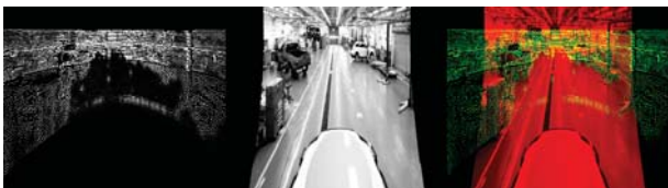
Fig. 5. Camera and velodyne scan being registered. Left, the velodyne scan. Centre, the Ladybug's centre camera image. Right the two sensor outputs overlaid.
