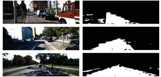
Fig. 5. The resulting output of our approach in perspective space. The first, second and third rows show the UU, UM and UMM category image respectively.
