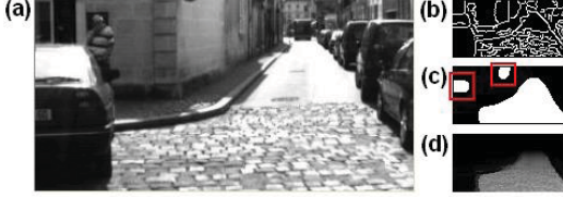
Figure 11. (a) Original image after sky removal and its Otsu's result in (c); (b) Canny edge detection result; (d) A multimodal 2D drivability free-area by considering the drag process.
