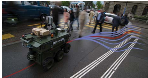
Fig. 1. ARTOR, a search and rescue robot specialized for outdoor applications navigating in highly dynamic urban environments. Typical mobile elements include pedestrians, bikers, cars, trucks and trams.
