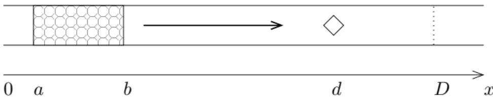
$$\begin{aligned} \partial_t \rho + \partial_x f(\rho) &= 0 & f(\rho(t, d)) &\leq q(\rho(t, d)) \\ \rho(0, x) &= \rho_0(x) & f(\rho(t, D)) &\leq Q(\rho(t, D)) \end{aligned}$$
