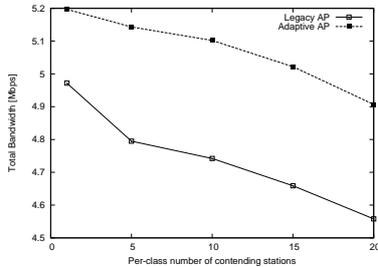
Fig. 5. Total bandwidth available in the network under the AW downlink scheduling, for two service classes ( $k_1 = 1, k_2 = 10$ ) compared with a legacy AP.
