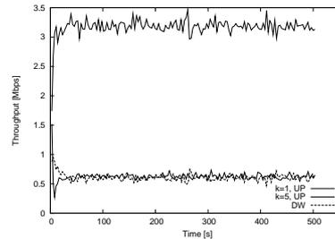
Fig. 3. Throughput repartition in case of heterogeneous application requirements ( $k_1 = 1, k_2 = 5$ ) for two contending stations under the AA downlink scheduling.
