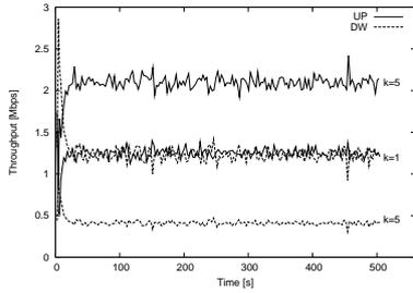
Fig. 4. Throughput repartition in case of heterogeneous application requirements ( $k_1 = 1, k_2 = 5$ ) for two contending stations under the AW downlink scheduling.
