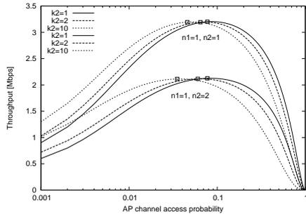
Fig. 2. Per-station total bandwidth, for different service classes ( $k_1 = 1, k_2 = 1, 2, 10$ ) and approximated maximum values (empty boxes).
