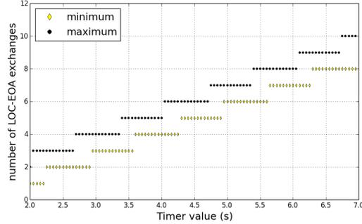
**Fig. 4.** Minimum and maximum number of LOC-EOA exchanges for  $O = 50$  ms, calculated through Eqs. (4) and (3).
