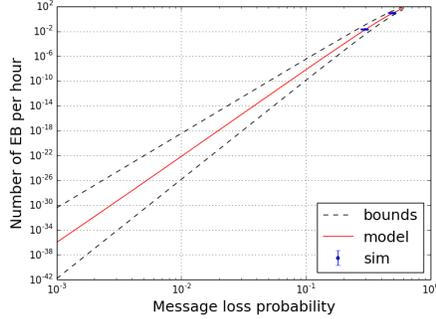
**Fig. 5.** Number of emergency brakes per hour when  $TM = 5.5$  s.
