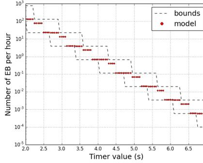
**Fig. 6.** Rate of emergency brakes when  $O = 50$  ms and  $p = 0.3$ .
