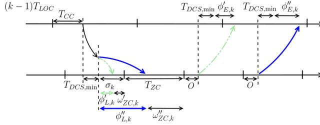
**Fig. 3.** Different delay components of the  $k$ -th LOC-EOA exchange for two different values of the LOC transmission delay  $\phi'_{L,k}$  and  $\phi''_{L,k}$ .
