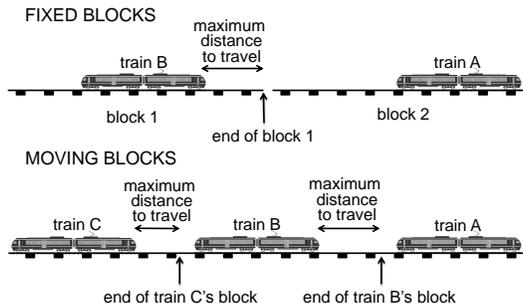
**Fig. 1.** Fixed-block and moving-block operation.
