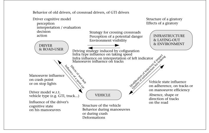
Figure 11. Model of the Driver-Vehicle-Infrastructure System.
